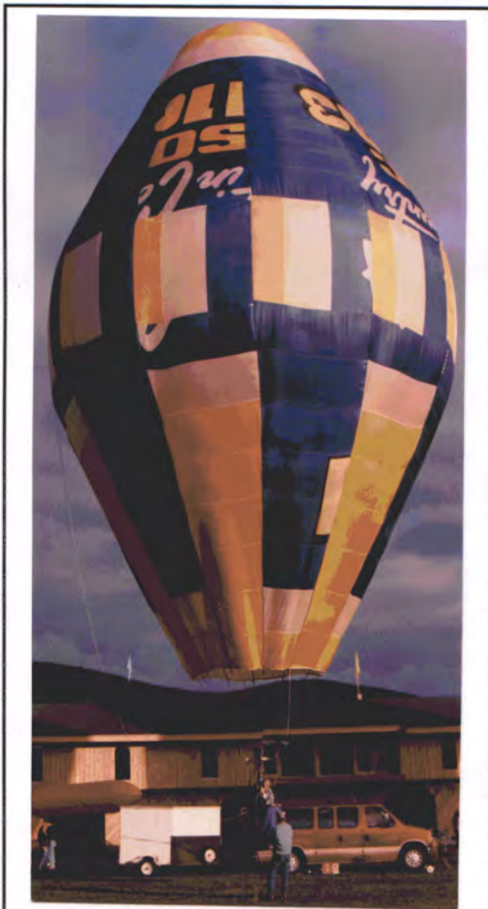
Figure 2: This two-day building project, affectionately called Conehead was reconstructed from an old envelope. The envelope was cut apart. The panels were turned around to put, what had originally been the fabric at the bottom of the envelope, up at the top.
